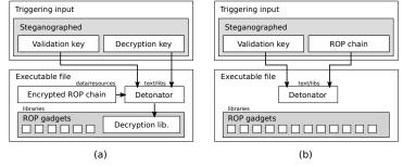
Figure 1: Implementation strategies: ROP chain embedded in (a) the executable file or (b) the input.
